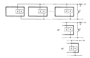
Note: H (Reset ON) level must be 4.5 V minimum.
